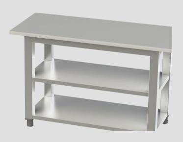
Frame structure in stainless steel AISI 304 fully welded 40x40mm tube, 1.00mm thick. 2 lower shelves welded to the structure. Top in white HPL 406/balck zodia 16mm thick, rounded R5 on corners. On adjustable feet.
