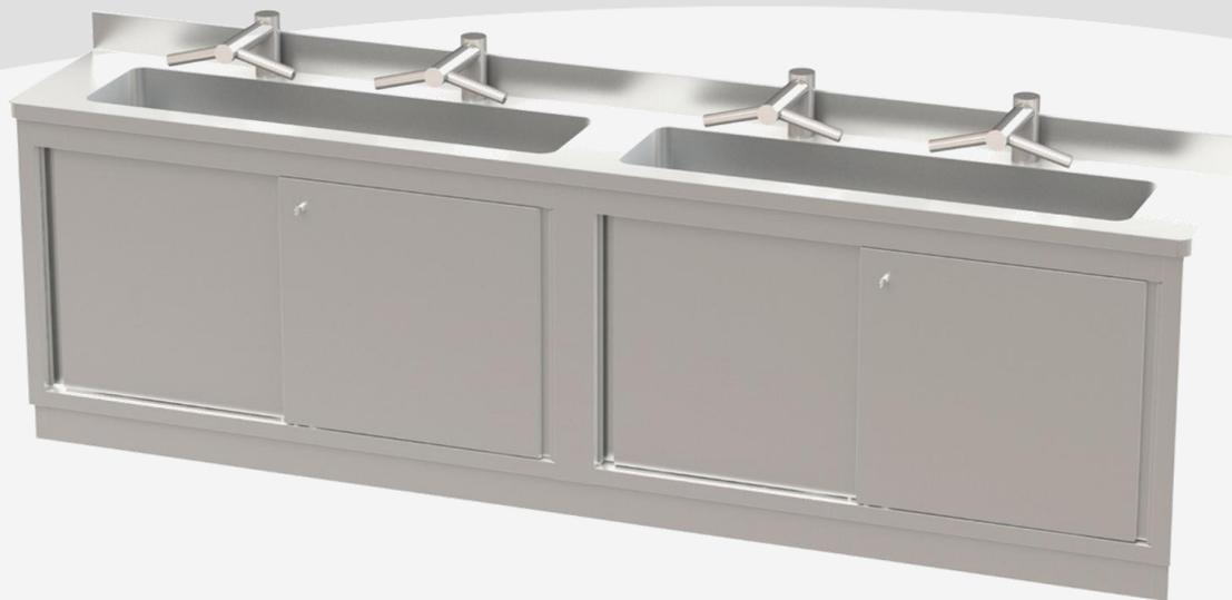
Made of AISI 304 Cr-Ni 18/10 stainless steel, Scotch Brite finish. Top with rounded R2 edges, and rounded R30mm front corners. No. 4 holes for Dyson mixer. Rear upstand H=100mm, welded and closed on the back. Sliding doors mounted on hygienic rails, easily removable without mechanical tools. Open back for hydraulic connections. PVC siphon, drain and stainless steel overflow included. Stainless steel supporting plinth advances on the back for rounded floor corner. Sink bowl dim. 1250x310x300Hmm.
