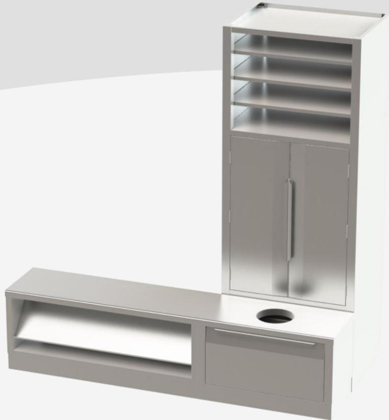
Step-over bench made of AISI 304 stainless steel folded sheet structure, Scotch Brite finish, on stainless steel supporting plinth H=100mm. On the left: compartment L=1200mm with double shoe holder welded to the structure. On the right: compartment L=800mm with drawer on stainless steel guides and hole on the seat for dirty clothes collection. Top in AISI 304 1.2mm thick with internal reinforcement and lower stainless steel infill. Long sides rounded R10.
