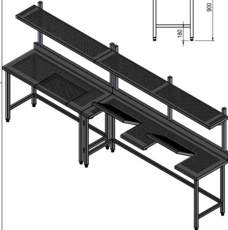
TAVOLO PER FLUSSO LAMINARE CON SPONDA POSTERIORE COMPLETA DI MONTANTI INTERNI E MENSOLA FORATA SUPERIORE P=350MM. PIANO CON NR. 3 PIANETTI A RIBALTA. ANGOLI POSTERIORI ARROTONDATI PER SGUSCIA R50. DIM. 3700X650X900Hmm
